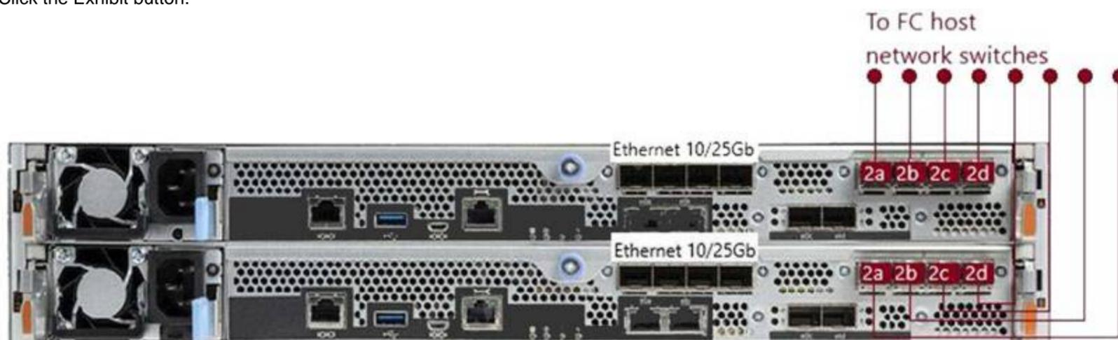
Referring to the exhibit, you installed a new AFF A250 HA system with FC at a customer site. The customer asks how many ports can be used for the Ethernet host connections. In this scenario, what would you tell the customer?
