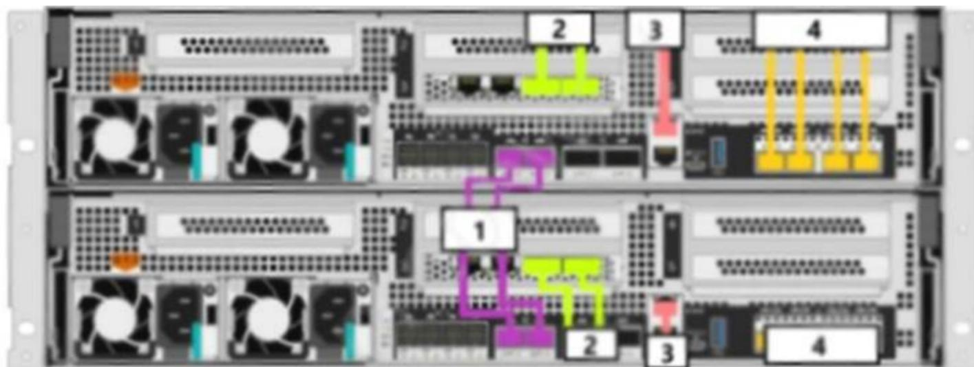
You want to add an AFF A400 system to an existing 4-node cluster. Referring to the exhibit, which number points to the ports that are used to cable the new nodes to the cluster interconnect switches.
