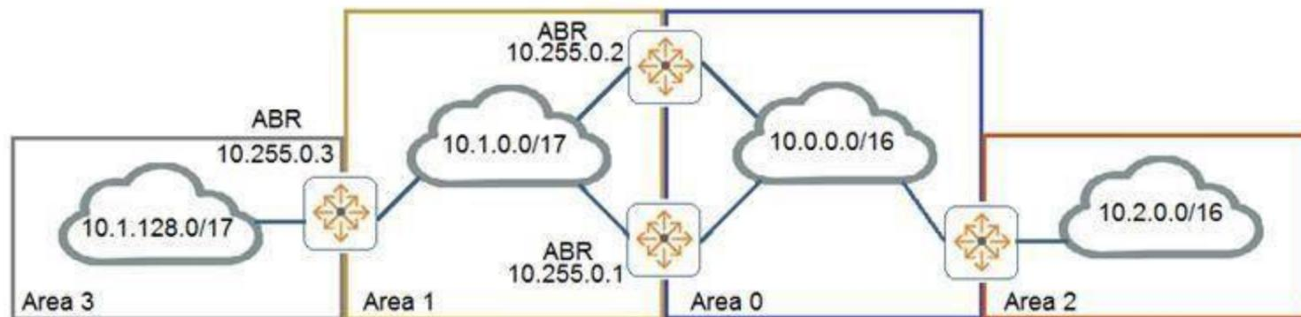
The network administrators is trying to add a remote location as area 3 to the network shown in the diagram. Based on current connection restrictions, the administrator cannot connect area 3 directly to area 0. The network is using AOS-CX switches. Which feature should the administrator implement to provide connectivity to the remote location?
