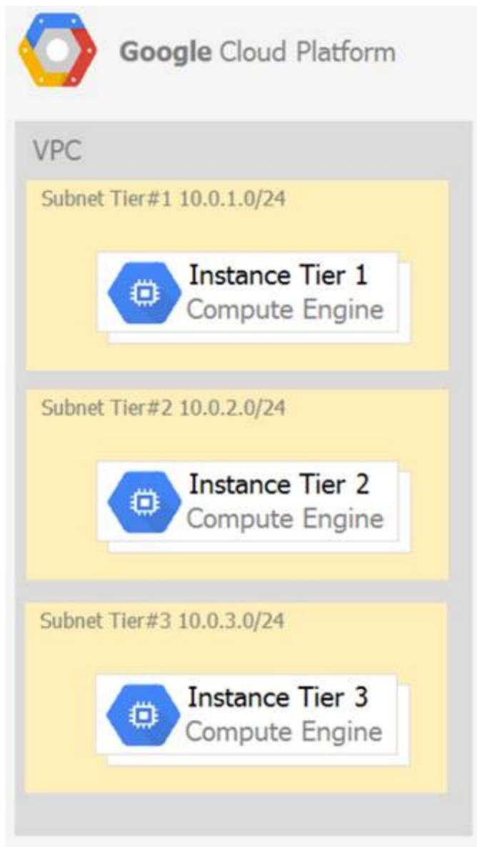
Each tier has a service account that is associated with all instances within it. You need to enable communication on TCP port 8080 between tiers as follows:
